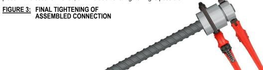
5) Fully assembled and installed FITT devices can be checked using the same pipe wrenches as described above. No additional tightening should be required. IT IS NOT NECESSARY TO USE A TORQUE WRENCH OR APPLY A HIGH TORQUE VALUE.
