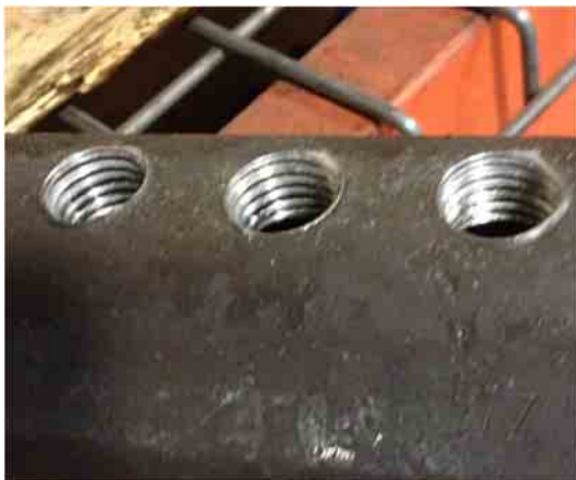
Figure 5. Clean Acceptable Coupler
