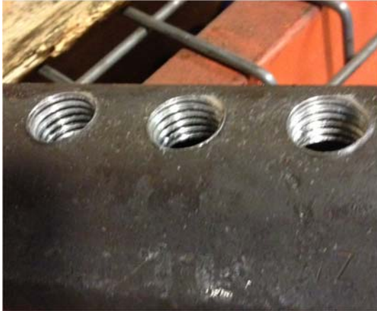
Figure 4. Clean Acceptable Coupler
