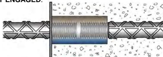
If the threaded rebar end does not properly engage into the Barsplicer coupler during assembly, stop immediately. Disassemble the connection to determine the problem. Possible causes of mis-assembly may be: mis-matched thread sizes; bars rubbing against each other; contaminated threads (i.e. concrete, dirt, etc.); or threads that have been damaged. Reassemble only after the problem has been identified and corrected.
