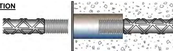
Just before assembly, check both internal and external threads for cleanliness. Clean off any foreign matter. **DO NOT USE CORROSIVE ACIDS.** Any thread damage must be corrected as noted above before installation.
