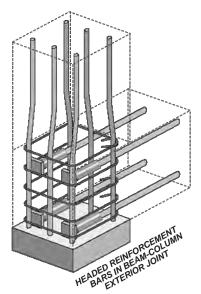
There are many situations in which the amount of space available is not sufficient to fully develop or anchor straight reinforcing bars subjected to tension. In the past, the most commonly used technique to reduce the required development length of bars subjected to tension was to terminate the bars using a 90 or 180 degree hook.
