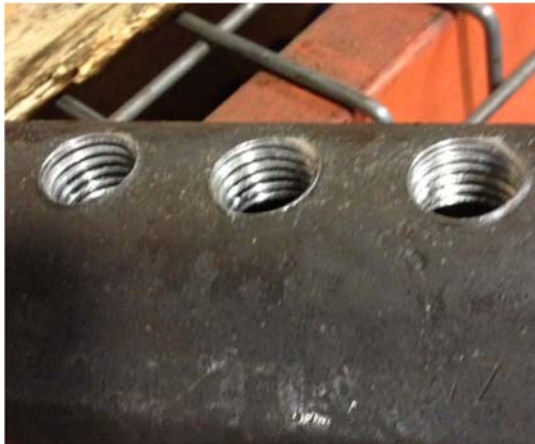
Figure 5. Clean Acceptable Coupler
