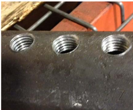
Figure 5. Clean Acceptable Coupler
